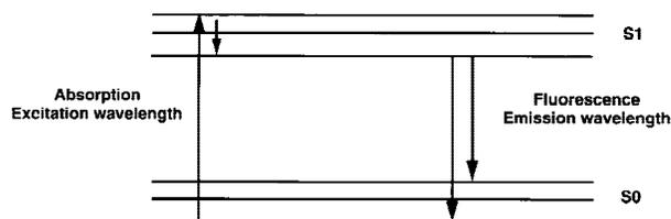
**FIGURE 1.** Jablonski diagram depicting the energy level transitions that occur during the process of fluorescence.
