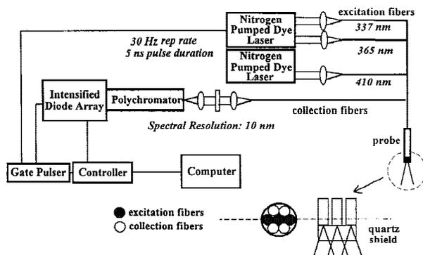
**FIGURE 2.** Schematic diagram illustrating one example of a fluorescence spectroscopy system designed for evaluation of tissue in vivo.
