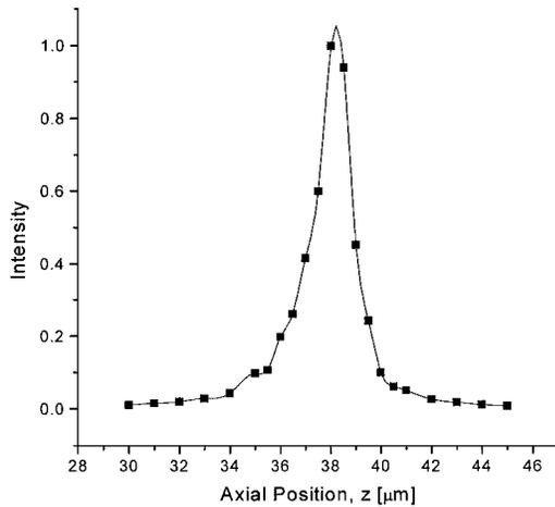
Fig. 3. Axial response of a plane mirror scanned through the focus. The FWHM is  $1.6 \mu\text{m}$ .
