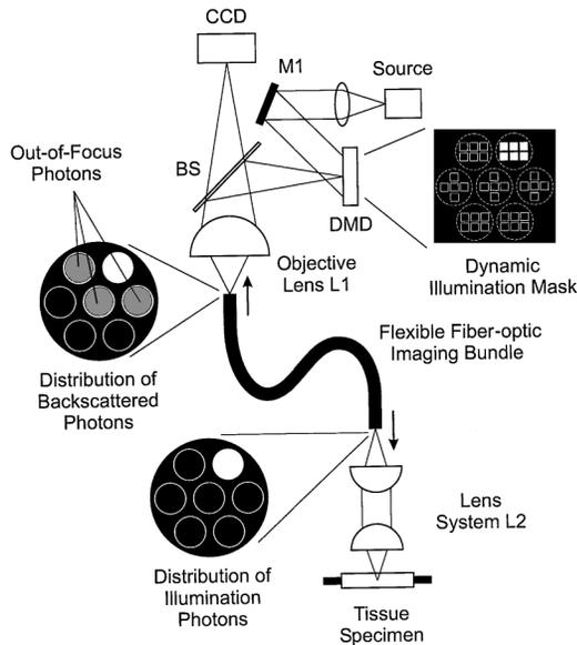
Fig. 1. Experimental setup. Individual fiber cores within the imaging bundle are illuminated by activation of an appropriate set of DMD mirrors. M1, plane mirror; BS, beam splitter.
