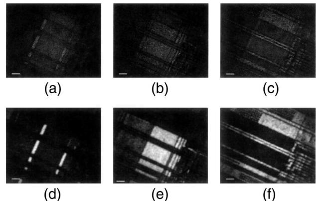
Fig. 2. Images of a Intel 486 microprocessor: (a)–(c) wide-field images at three different focal planes, (d)–(f) confocal images at the same levels. The scale bars are 10  $\mu\text{m}$ .
