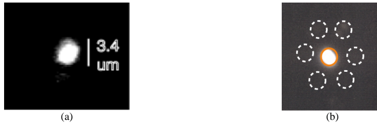
Fig. 4. Part (a) shows the focal spot formed by the telescope/scan lens system. The spot diameter is approximately 3.4\ \mu\text{m} . Part (b) shows the distal end of the fiber bundle when only one fiber is illuminated by the telescope/scan lens. Dotted circles represent the surrounding fibers.
