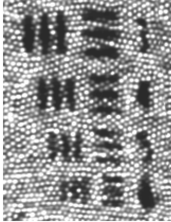
Fig. 7. Image of resolution target taken with the fiber confocal reflectance microscope. The smallest features have line thickness and spacing of approximately 2\ \mu\text{m} .
