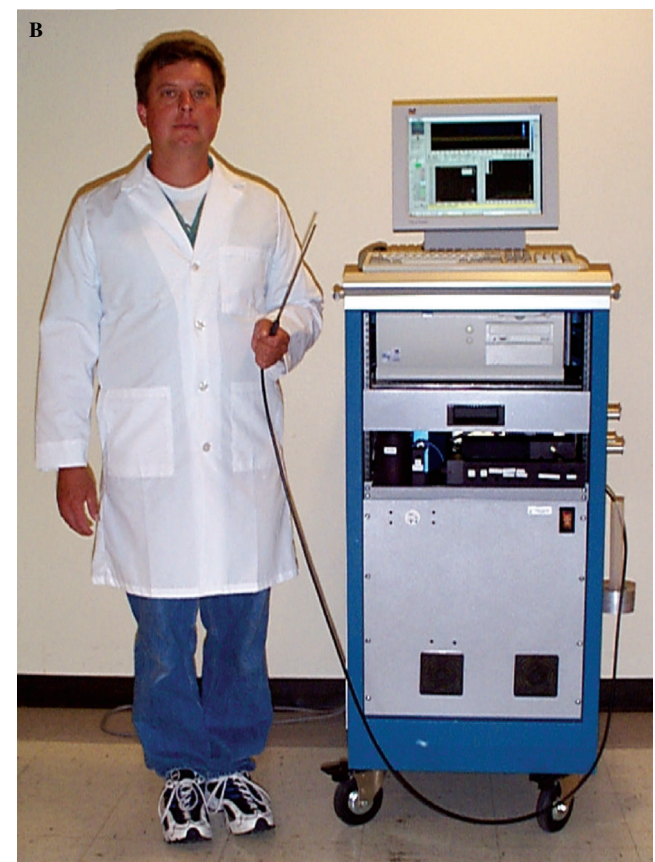
Fig. 3. A) This is a system block diagram or cartoon showing an excitation light source assembly, a fiber-optic delivery system and collection probe, and a polychromator assembly; B) A photograph of the actual device built by our laboratory and being used in the clinic for the pilot trial.
