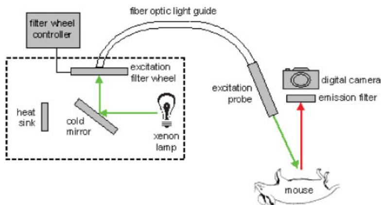
Fig. 1. Schematic of macroscopic fluorescence imaging system. Light from a Xenon arc lamp is directed by mirror to the excitation filter wheel with a bandpass filter centered at 545 nm. Excitation light enters a flexible fiber optic light guide for delivery to the mouse. Fluorescence emission from the mouse is recorded using a digital SLR camera fitted with two emission filters, a bandpass filter centered at 610 nm and a 570 nm longpass filter.
