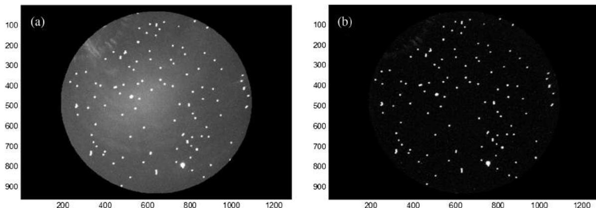
**Fig. 12** Images taken with the miniature microscope from the (a) classifier 1 channel and (b) classifier 2 channel at an exposure time of 300 ms. Note that due to filter spectral characteristic, classifier 1 channel exhibits stronger background signal.
