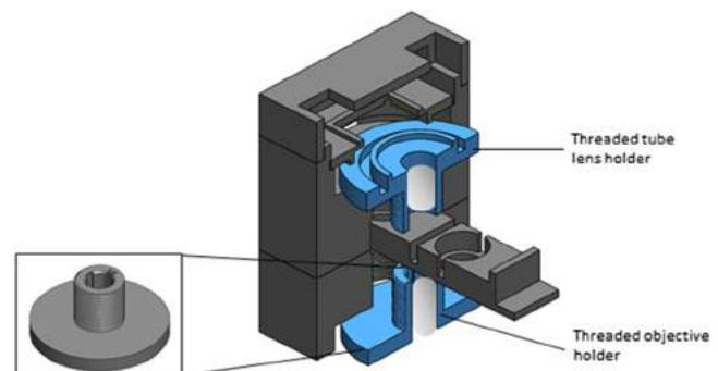
**Fig. 9** A cross-section of a Solidworks rendering of the miniature microscope is shown above. The rendering illustrates an exploded view of the system cross section highlighting the threaded objective and tube lens holders. The inset image shows an enlarged view of the threaded objective holder.
