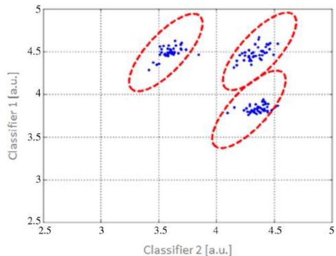
**Fig. 16** A bead map from a multiplexed bead sample imaged on the miniature microscope. The sample contains 137 total beads composed of three distinct bead types, which can be resolved into three distinct groups (outlined with red ellipses). Each group is spaced ~0.6 units apart in the y-direction and 0.8 units apart in the x-direction.
