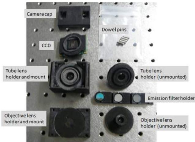
**Fig. 10** The disassembled infinity-corrected miniature microscope components (camera cap, camera mount, objective mount, tube lens mount, and emission filter holder). Examples of the 3/10 dowel pins (Brikksen, Germany) used to connect the modules are shown in the top right corner. Dowel pin holes are visible on the tube and objective lens modules. Extra unmounted tube lens and objective lens modules are shown to the right of the microscope.
