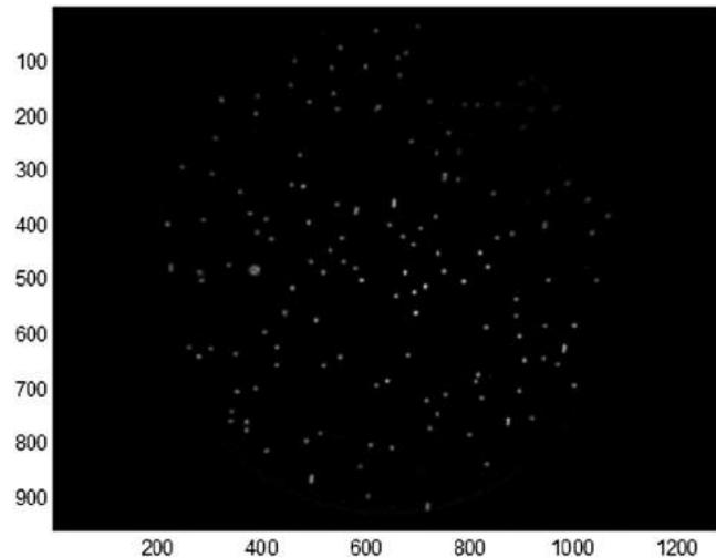
Fig. 14 An example of a postprocessed HDR image from the reporter channel of bead 39 tagged with  $10^{11}$  copies of DNA (detailed description of image processing operations in the main text). Please note beads intensity variations, caused by difference in concentration of target analyte.
