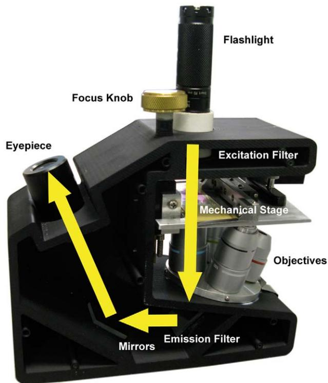
**Figure 1. The Global Focus microscope.** In this schematic, yellow arrows indicate the trans-illumination light path of the Global Focus microscope.
