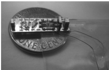
Fig. 3 Assembled 4M device shown above a United States penny for scale. The system incorporates the micromounted lens, hybrid printed lenses, beamsplitter, illumination optics, and fiber holder. The image is formed at the location where the detector will be integrated in future devices. This intermediate image is relayed by optical bench relay lenses to a CCD camera for testing purposes.
