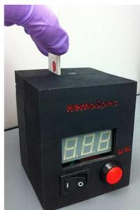
We investigate using chromatography paper as a low-cost medium for spectrophotometric assessment of blood hemoglobin concentration and present a prototype low-cost reader for field evaluation.
