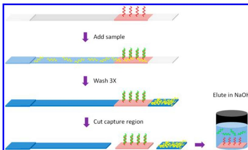
**Figure 1.** Lateral flow-based enrichment of target DNA. Capture oligonucleotides are shown in red, target DNA is shown in green, and background DNA is shown in yellow. Target DNA binds to the capture oligonucleotides, background DNA is washed away, the capture region is excised, and target DNA is eluted.
