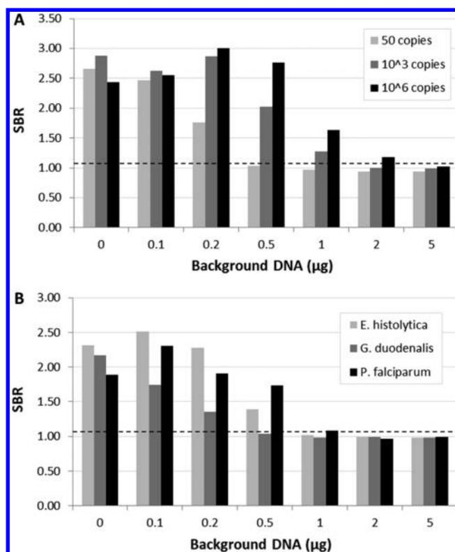
**Figure 2.** RPA inhibition by background DNA. (A) Results of lateral flow assay to detect RPA products in reactions with different amounts of HIV-1 target DNA and background DNA. (B) Results of lateral flow assay to detect RPA products in reactions with 1000 copies of target DNA and various amounts of background DNA for three different assays. The threshold for positive samples (1.05) is shown by the black dashed line.
